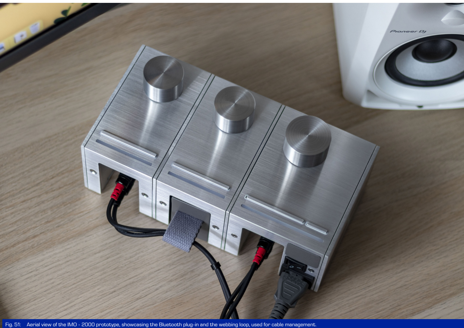
Fig. 51: Aerial view of the IMO - 2000 prototype, showcasing the Bluetooth plug-in and the webbing loop, used for cable management.
