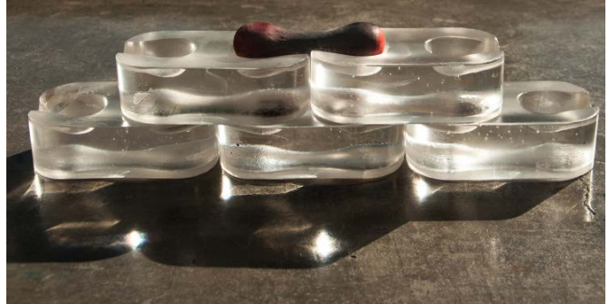
Fig.4: Type A blocks: Column (left) and wall (right) configuration
