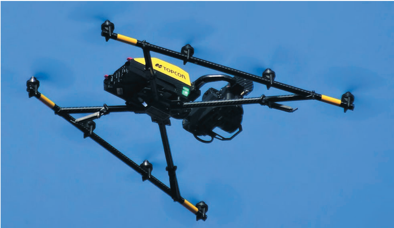
▲ Figure 2: UAS equipped with camera as tool for cadastral boundary survey (courtesy: M. Lemmens).
