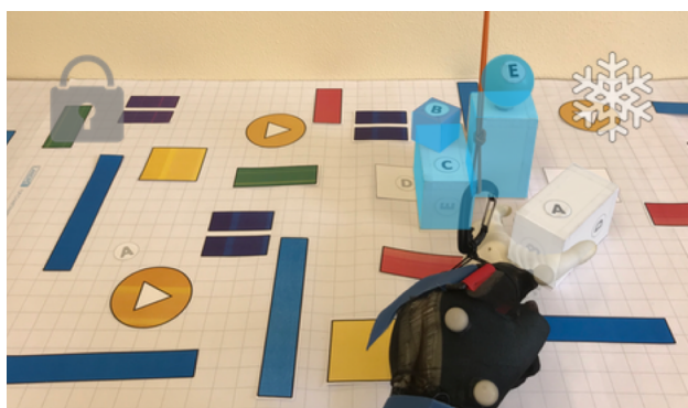
Figure 9 | Workflow Step 5. The user is almost touching the object. The prosthesis is frozen. The Prosthesis Frozen state icon is visualized and the object turns white.
