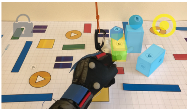
Figure 6 | Workflow Step 2. The system infers user intention to grasp object C from the front/side. The object assumes a yellow-green texture, the prosthesis is preshaped, and the Scene Locked state and Prosthesis Preshape state icons are displayed.
