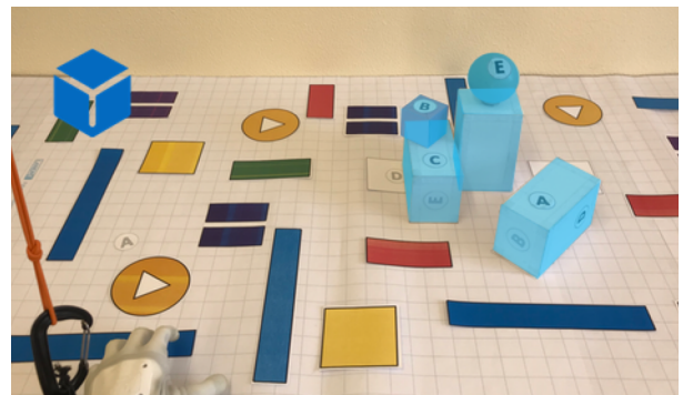
Figure 5 | Workflow Step 1. The objects in the scene are modeled and blue holograms are presented to the user. The top-left icon indicates the system is in Scene Modeling state.
