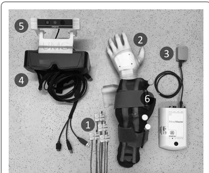
Figure 2 | System components. The system comprises (1) eight dry surface EMG electrodes, (2) a prosthesis with two grip types, active wrist and flexor, (3) an inertial measurement unit, (4) augmented reality glasses, (5) a color and depth camera, (6) three retroreflective markers and a standard PC (not illustrated in the figure).
