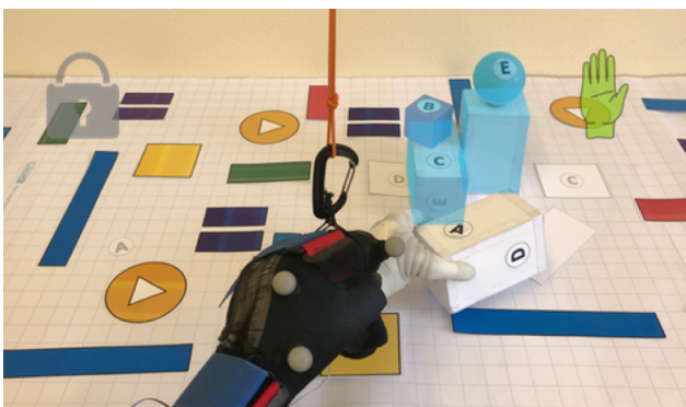
Figure 11 | Workflow Step 7. The user grasps an object. The corresponding hologram is destroyed.
