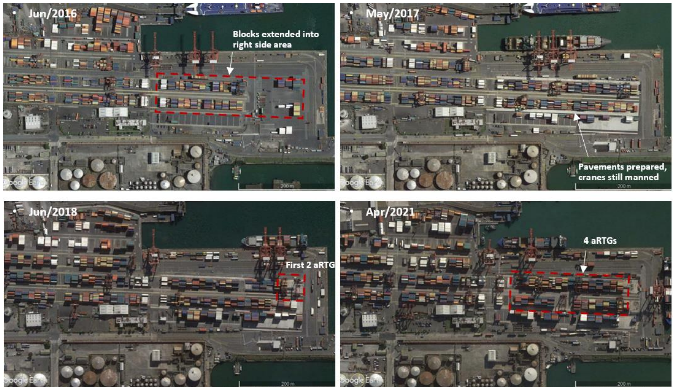
Figure 5-5: implementation process of new aRTG stacks in the CT N°50, Dublin, Ireland.
