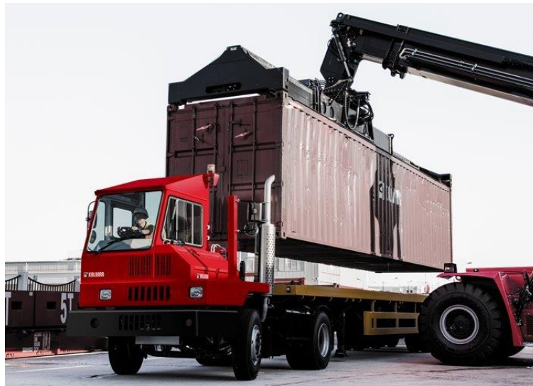
Figure 2-6: TT attached to a chassis during the transfer of a container 6 .
