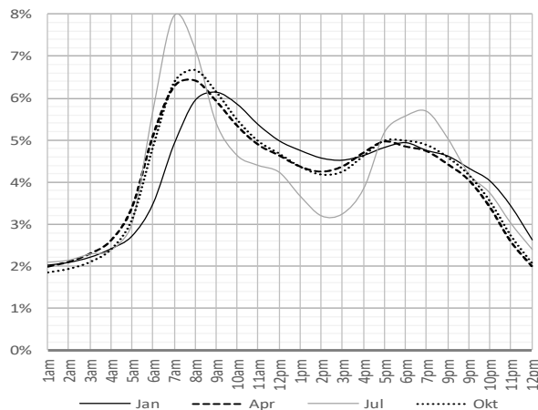
Figure 5.2 For exemplary purposes: 24 h gas demand curve for an average household in NL, based on Liander data. The % represents the demand for that hour relative to the daily total. Two peaks are evident for each of the four curves: a morning peak when people wake up, turn on the heat-ing and have a shower and an afternoon peak, when people tend to cook dinner (on gas stoves) and switch on the heating (again).
