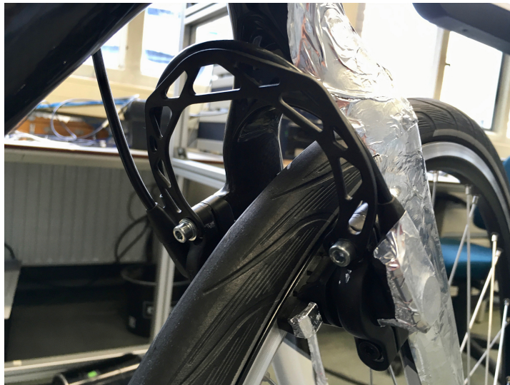
Figure 2.18: Magura brake system with a brake booster.
