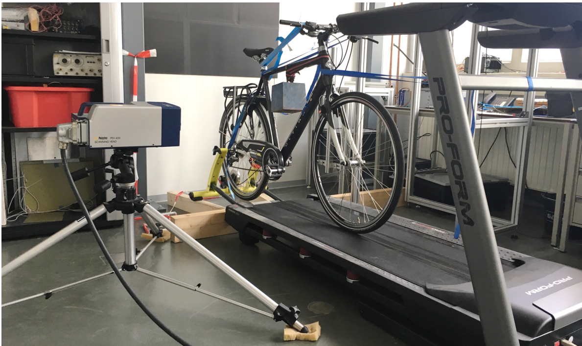
Figure 2.10: Experimental setup to perform measurements with the laser doppler vibrometer.
