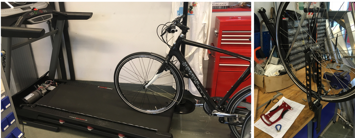
Figure 6.1: The setup for this experiment (a). A wheel truing stand is used to adjust and measure the spoke tension (b).
