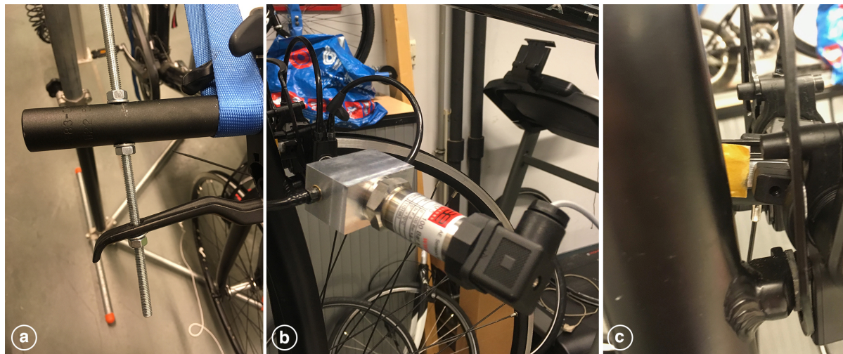
Figure 5.5: Brake lever connected to handle bar with threaded rod (a), fluid pressure sensor connected to the brake system and movement of the wheel is made visible with a little reference sticker attached to the rim (c).
