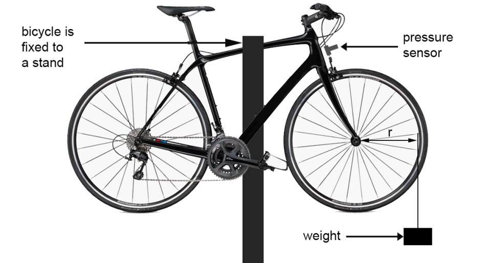
Figure 5.1: The experimental setup to measure the friction coefficient of various types of brake pads.
