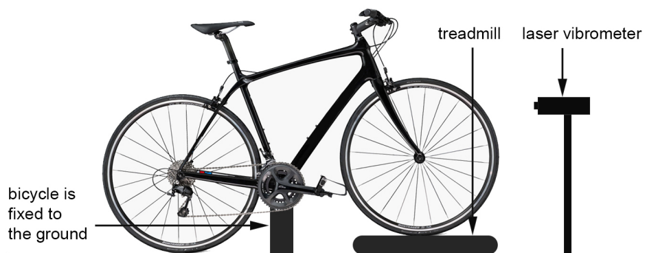
Figure 2.9: Experimental setup to perform measurements with the laser doppler vibrometer.
