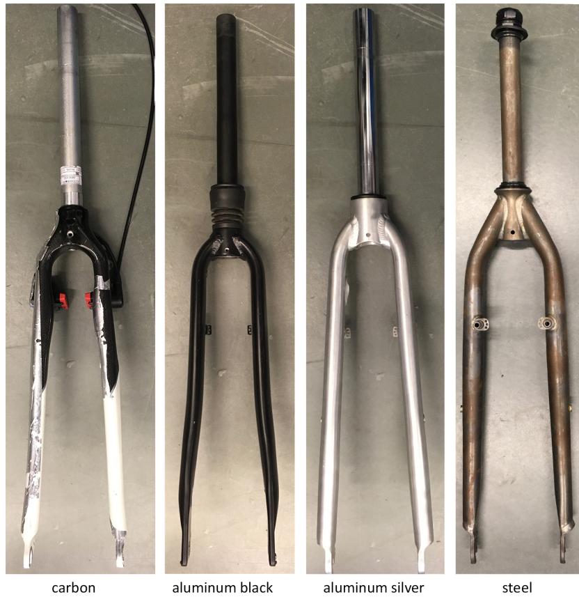
Figure 4.4: The four different front forks that will be used in this experiment
