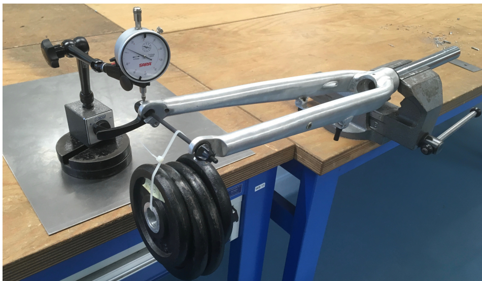
Figure 4.5: Experimental setup to measure front fork bending stiffness
