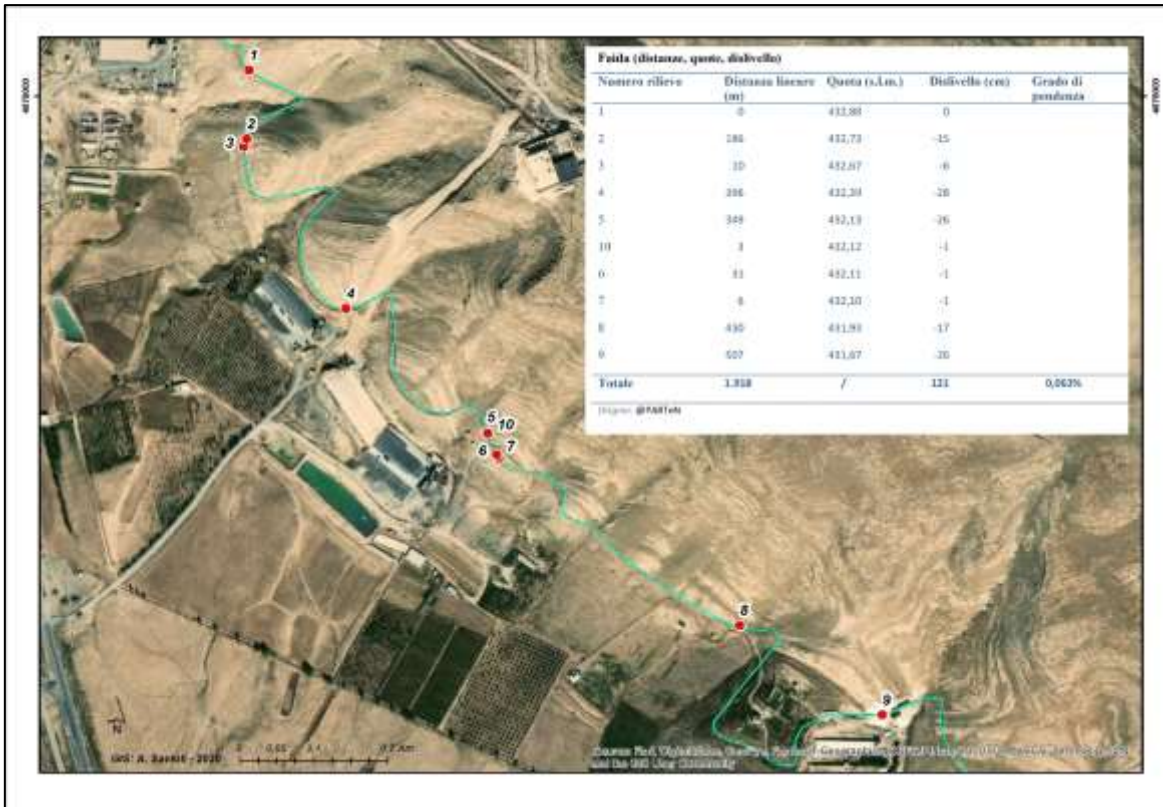
Figure 4 Bed slope data from LoNAP team, with slopes ranging from 0,5 to 0,7 m/Km in reaches containing offtakes.
