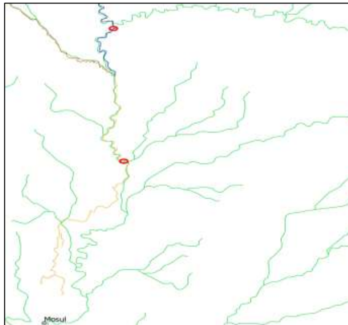
Figure 41 Khosr and Kisiri reaches with nearby settlements, streams crossing them (green) and input locations (red).
