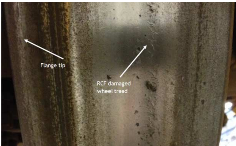
Figure 1. Wheel tread with RCF crack damage.
