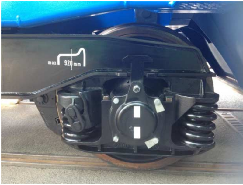
Figure 3. Y-25 primary suspension consisting of a set nested coil springs and a single Lenoir link.
