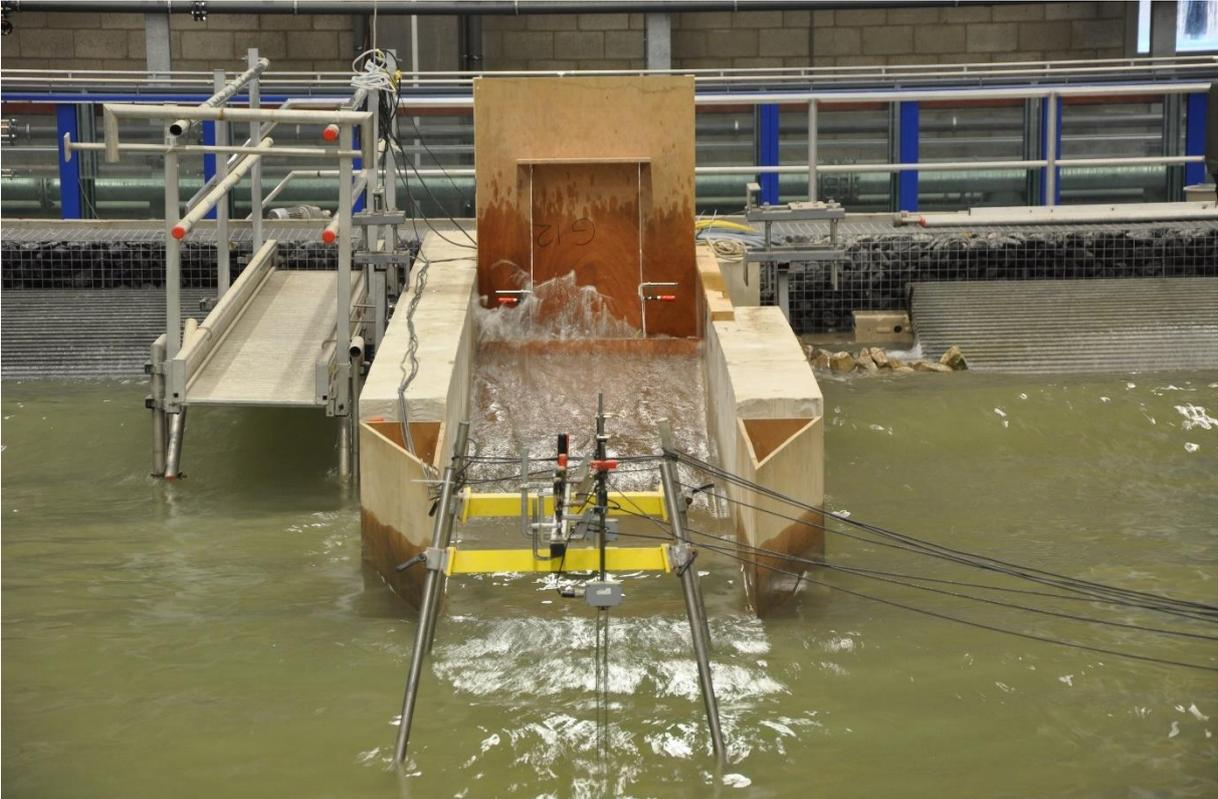
Figure B.6: Front view with the three wave gauges measuring the wave height and period in front of the dike; dike configuration with a crest wall.
