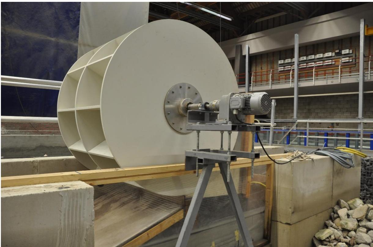
Figure B.3: Side view; dike configuration with a crest wall with paddle wheel.
