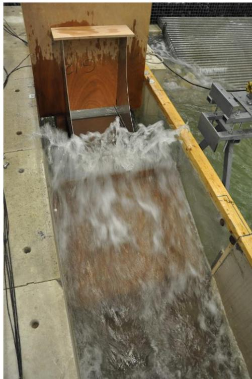
Figure 3.2: Vertical splashing of water when waves hit the crest wall on the dike with crest wall only.
