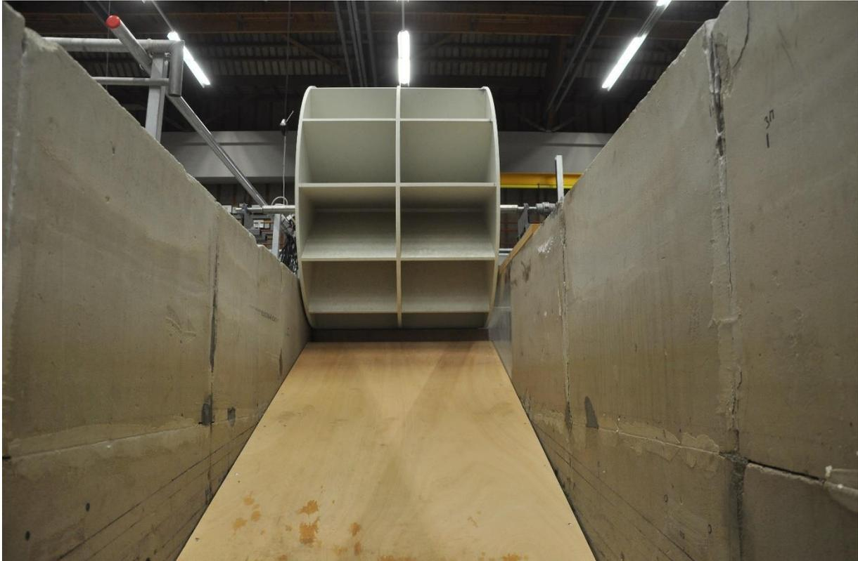
Figure B.2: Front view; dike configuration with a crest wall and promenade with paddle wheel.
