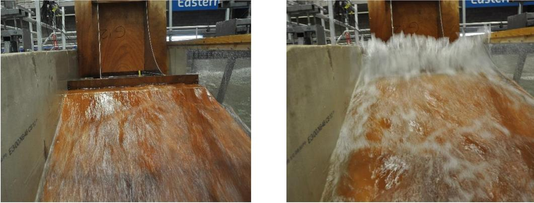
Figure 3.3: Vertical splashing of water when waves hit the crest wall on the dike with crest wall and promenade.
