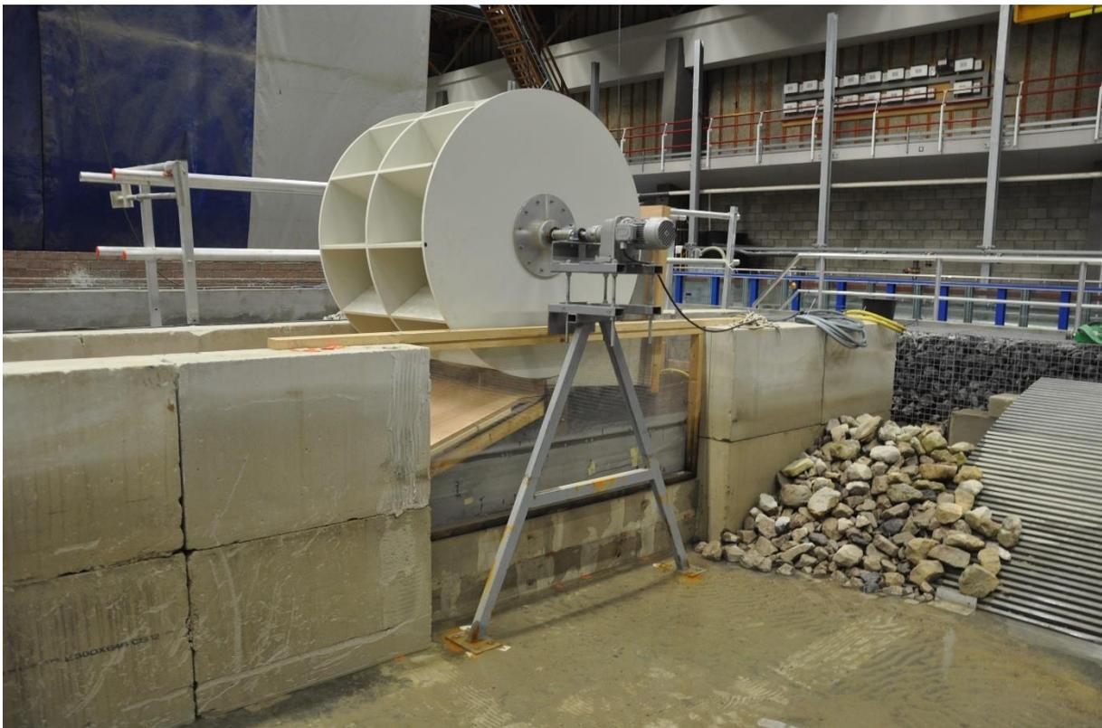
*Figure B.1: Side view; dike configuration with a crest wall and promenade with paddle wheel.*
