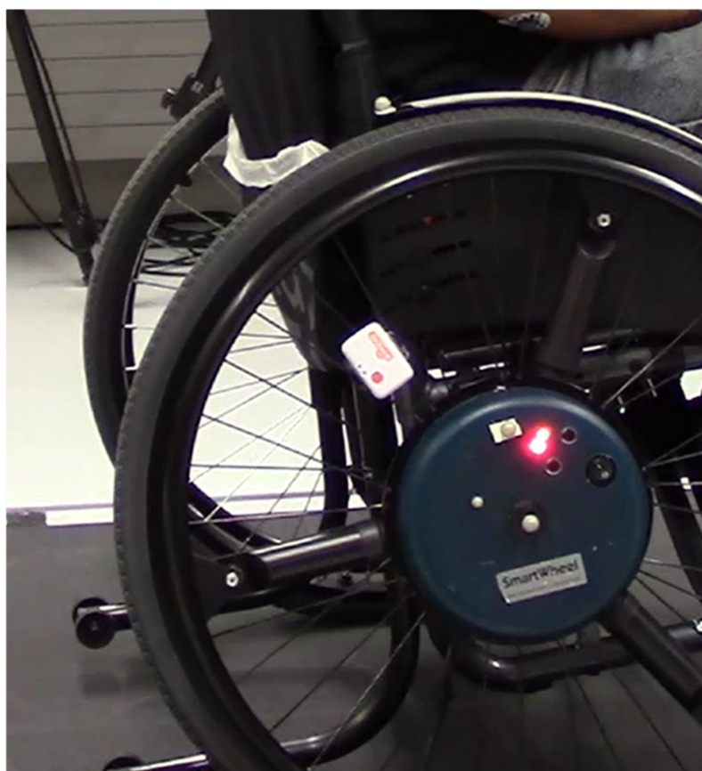
Figure 1. Equipment used. A standard active wheelchair with a Smartwheel on the right side, a Shimmer IMU attached to the wheel in such a way it did not hinder propulsion and another IMU attached to one of the horizontal bars of the wheelchair frame (not visible here).
