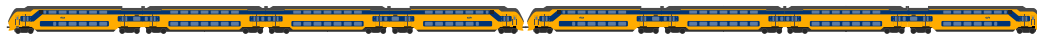
Figure 2.1: An example train or shunting unit consisting of two VIRM train units, with 4 carriages each. Illustration from Wikimedia 1 .
