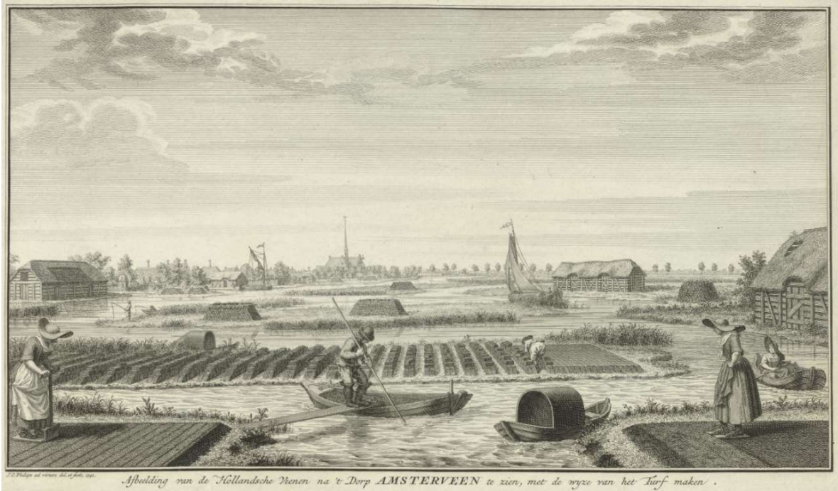
Figure 6: Peat mining by dredging circa 1742 (Jan Caspar Philips, Rijksmuseum Amsterdam). Peat is dredged using a “didle” 19 ( baggerbeugel ), spread on the land, and stamped down. When it is firm enough, it is cut into turves, which are then stacked to dry. In the background the final product is transported to the market. In a later stage the remaining strips of land would be cut.
