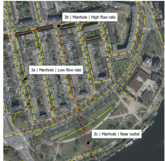
(b) Manhole locations and flow rates during a standard design event (Bui02)
