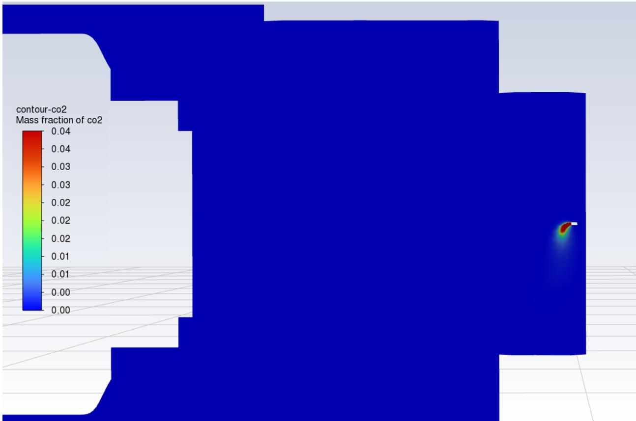
**Figure 5.26:** Contour of carbon dioxide concentration in the vicinity of the vacuum tank of CMS in its open configuration (fitting leak case). There is no threat to workers in the cavern, with the leakage spreading about a meter from the leakage point.
