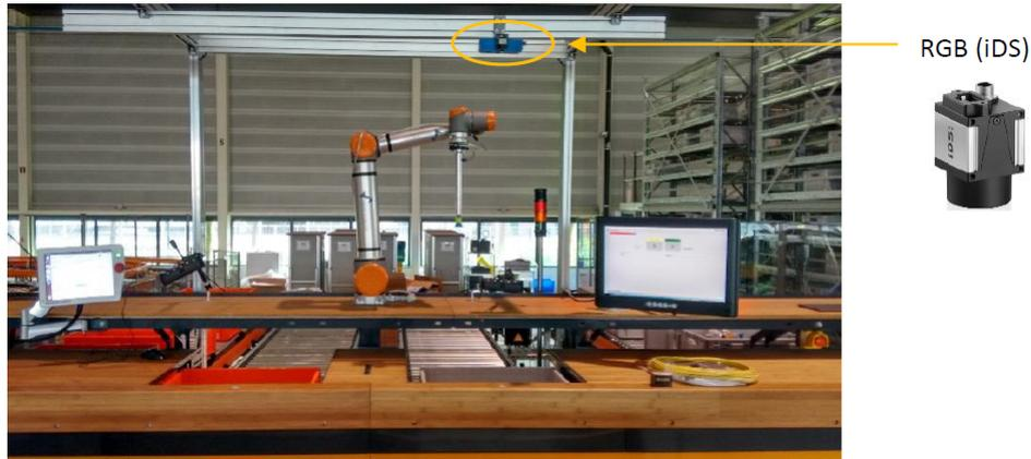
**Figure 5-4:** Data collection configuration. Container images are taken from the top side with an RGB camera. Items in the containers are placed and repositioned manually.
