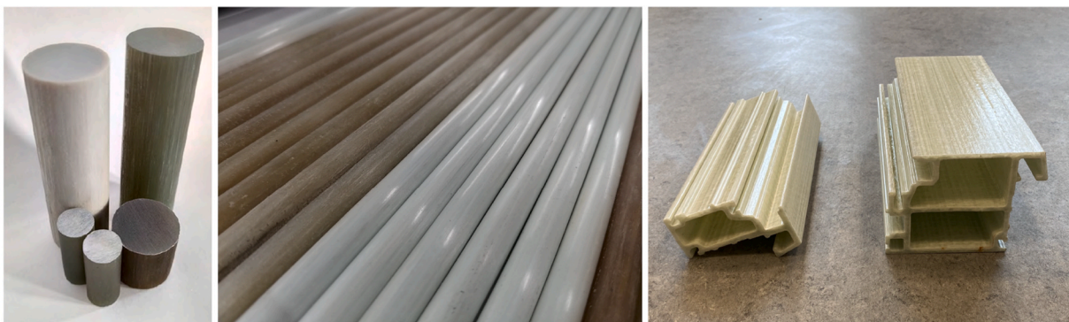
Fig. 1. Fibre-reinforced, thermoplastic rods with different diameters (left and middle, \varnothing 10 - 40 mm), fibre-reinforced, thermoset profiles with complex cross sections (right, w \times h \approx 60 \times 60 mm 2 , wall thickness 2 mm). All these profiles were manufacturing using the pultrusion process.
