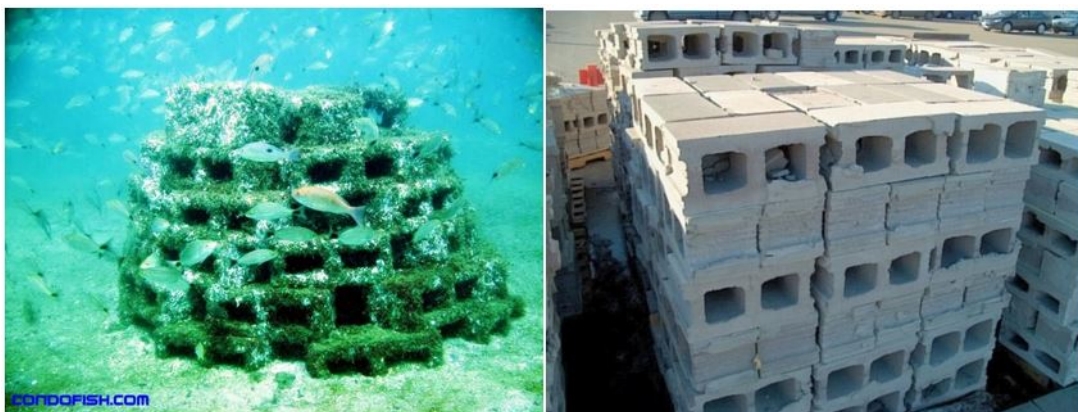
Figure 7.6: Hollow cinder blocks applied in a marine environment.
