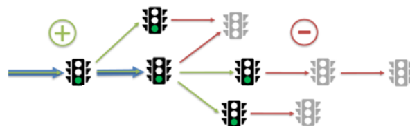
Figure 1-4: The service increase outflow . Traffic lights give more green resulting in better traffic conditions in front of the traffic light. The traffic condition of the roads after the traffic light deteriorates. [Technolution]
