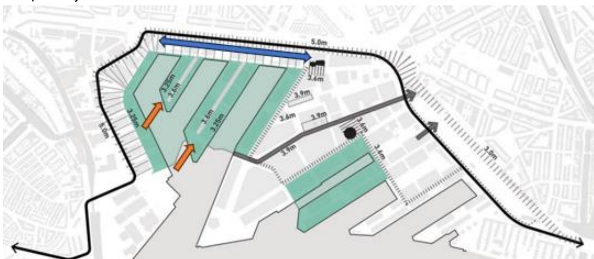
Figure 23: Visualisation of the main concept choices in the adaptation strategy. Green: 'living with water' and white: 'keep water outdoors'. The black arrow and the green arrows visualise the evacuation routes, blue arrow points out Marconistrip and the red arrows point out the Merwepieren (Adapted from Van Der Visch et al., 2019).
