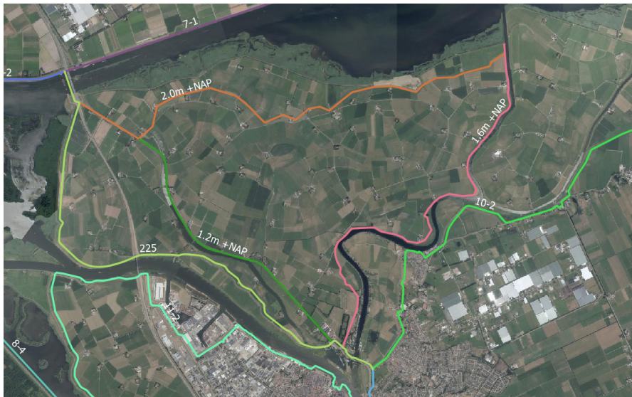
Figure 4.6: Crest heights of the two main compartments inside the Kampereiland. Heights obtained from [16].
