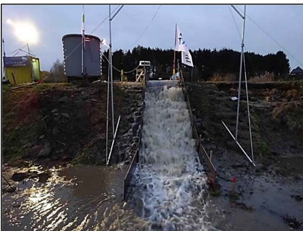
Figure 6. Observed aerated flow during the overflow experiment
