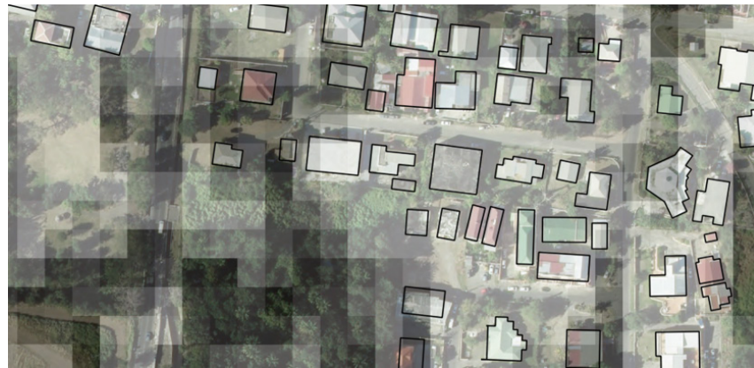
Figure 4.9: SAR coherence map superimposed on buildings [Based on: RescUAV (17 Sept. 2017), Middle Region - Sint Maarten [georeferenced image], used under CC-BY4.0 as part of Open Imagery Network, retrieved from www.openaerialmap.org ]
