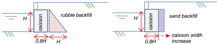
Figure 3.3. Design choice: rubble backfill or increased caisson width
