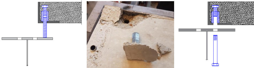
Fig. 4. a) Rod acting as support (3); b) Punched connector (top view) (3); c) Construction method using long bolts (3)
