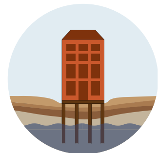
Lowering of the groundwater level, wooden foundations get dry, leading to rotting poles
