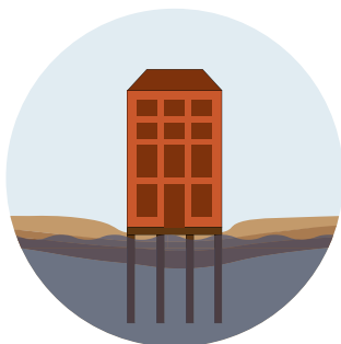
Subsidence because of peat oxidation and compression by the weight of the city, groundwater level relatively high
