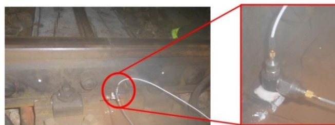
(a) Accelerometers used to measure impact vibration
