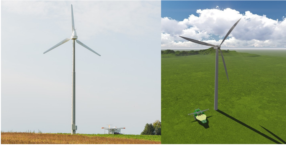
Figure 1.2: Comparison of conventional wind turbines to AWE systems with similar rated power output: The left picture shows the TwingTec prototype [107], the right picture shows a rendering of AP4 which has a rated power of 2 MW and is designed by Ampyx Power [90].
