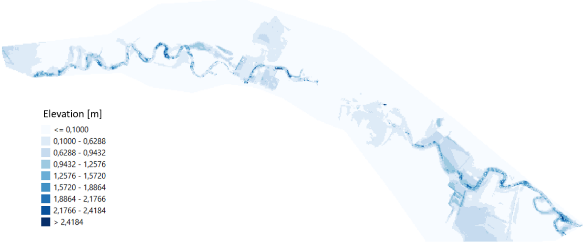
Figure B.4: Individual water depth results for ten-year precipitation event used to create the flood extent map for Valkenburg
