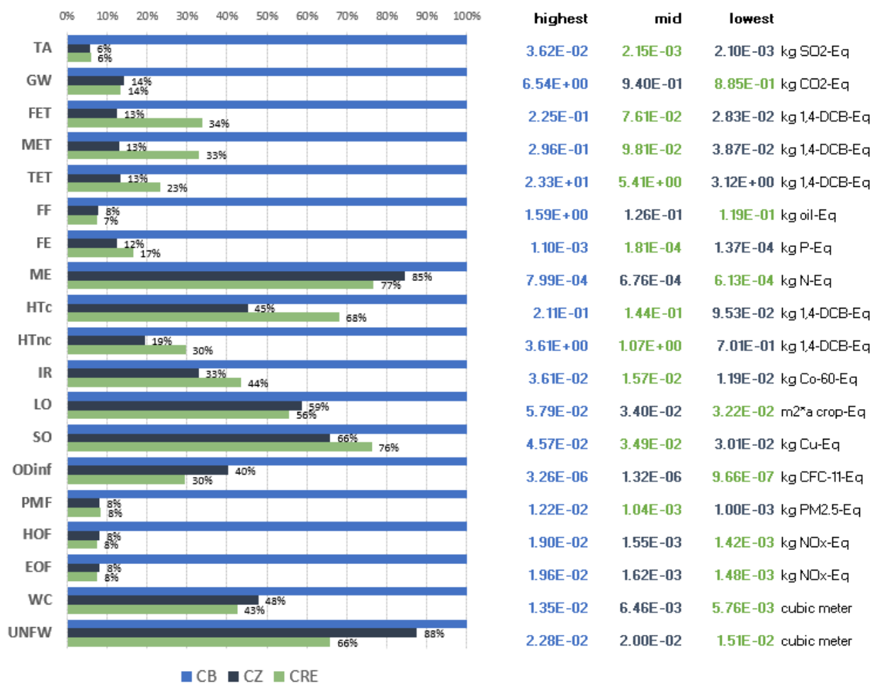
Figure 11 Environmental profile comparison, CB vs CZ vs CRE. Adjusted to the highest score.
