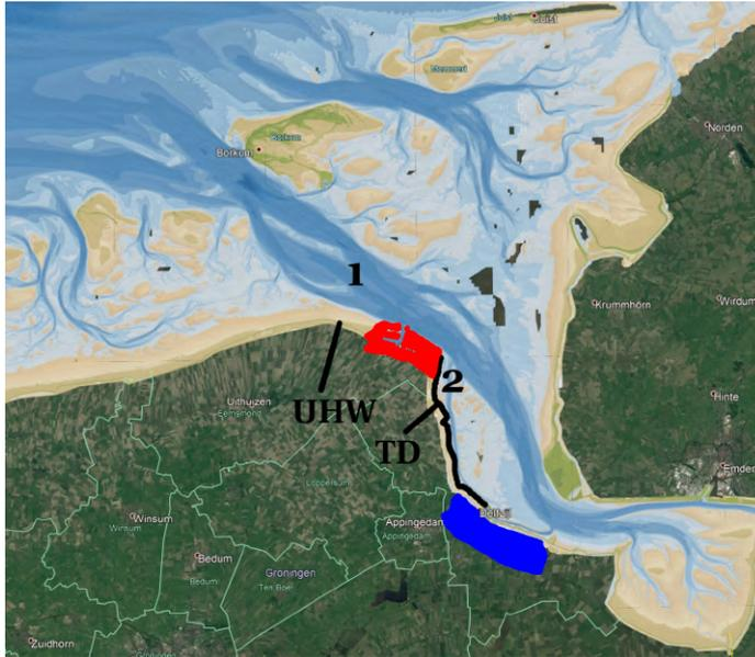
Figure 1.2: Eems-Dollard estuary, with the port Eemshaven (red area), the town Delfzijl (blue area), the deep main tidal channel (number 1), the secondary channel the Bocht van Watum (number 2), the dike section of interest (black line) and the two locations of interest for the field measurements, Uithuizerwad (UHW) and the Twin Dikes (TD). Bathymetrical data from Rijkswaterstaat six-yearly bathymetrical surveys, blue is deeper, yellow is shallower.
