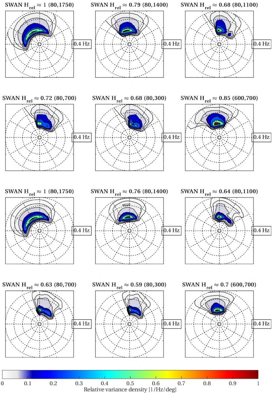
Figure 4.19: 2D SWAN spectra at several locations. First two rows: SWAN with WBI settings, with wind imposed. Bottom two rows: SWAN with recommended settings, diffraction approximation, 20 m grid cells and with wind. Variance density normalised and colour-scaled with the maximum variance density at the offshore (80,1750) location.
