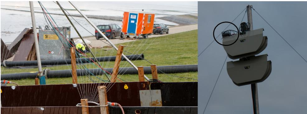
Figure 5.3: Left: Simulation of rain with garden sprinklers. Right: Laser scanners with guywires and accelerometer (circle).
