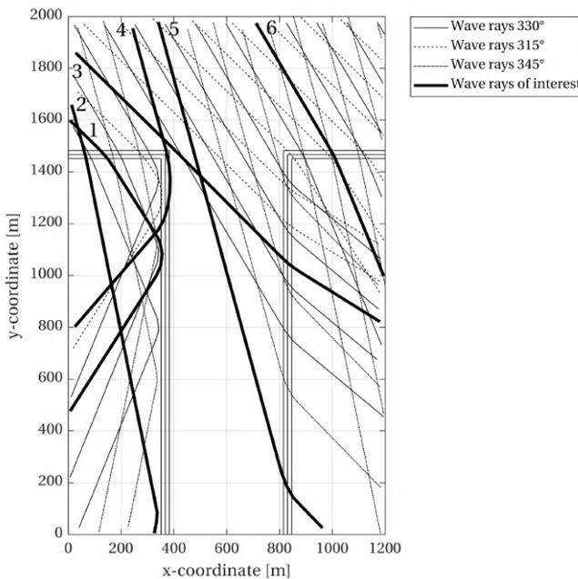
Figure 4.15: REFRACT wave rays for the detailed model. The mean wave direction and 30° directional spreading are represented by wave rays from 330°N, 315°N and 345°N. Several wave propagation effects occur: Relatively unaltered propagation onto shallow flats (2 and 6), relatively unaltered propagation into channel (5), wave defocusing on channel slopes (4), refraction out of channel (3), and wave reflection off the channel slope or wave trapping (1).
