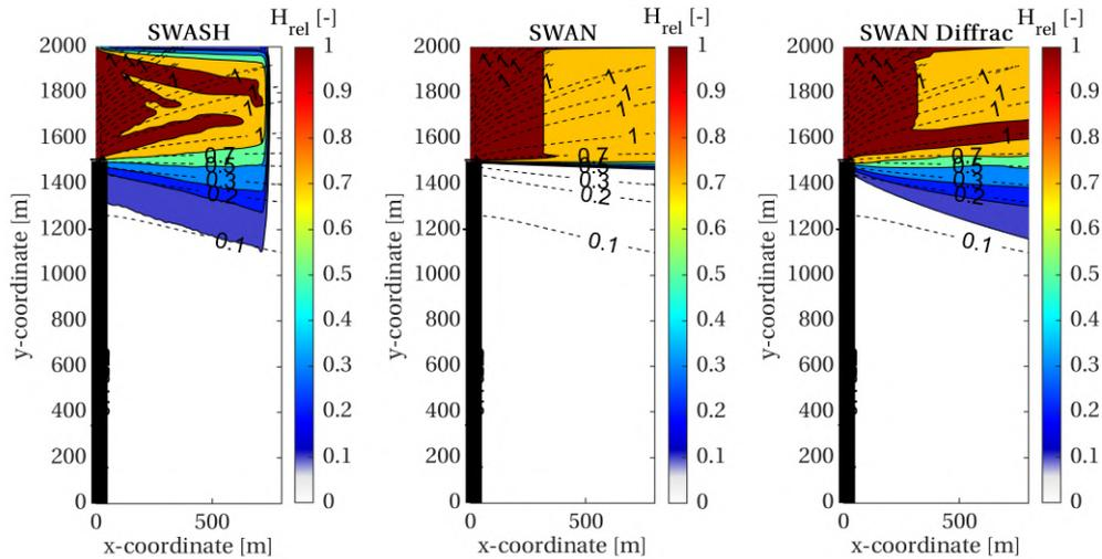
Figure 4.9: Diffraction for semi-infinite breakwater case with irregular, narrow-spread waves coming from 270°N. SWASH (left), SWAN with recommended settings (middle) and SWAN with recommended settings, diffraction approximation and 20 m grid cells (right), compared to analytical solution of Penney et al. (1952); Sommerfeld (1896) (black dashed lines). The thick black line indicates the dike.
