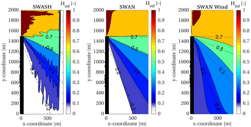
Figure 4.12: Diffraction for semi-infinite breakwater case with irregular, broad-spread waves coming from 270°N. SWASH (left), SWAN (without diffraction approximation) without wind imposed on the model (middle) and SWAN with wind imposed (right), compared to analytical solution of Goda et al. (1978) (black dashed lines). The thick black line indicates the dike.
