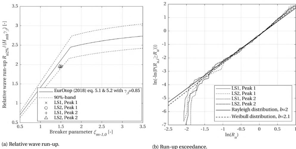
Figure 7.10: Left: Relative wave run-up versus breaker parameter. Figure based on EurOtop (2018). Note the added influence of the oblique wave attack on the vertical axis compared to EurOtop (2018). Data for both laser scanners based on measured distances, and for both storm peaks. Right: Run-up exceedance plots for both laser scanners and both storm peaks, plotted on Weibull scale. A straight line gives a Weibull distribution, a straight line with a slope of 1:2 gives a Rayleigh distribution.
