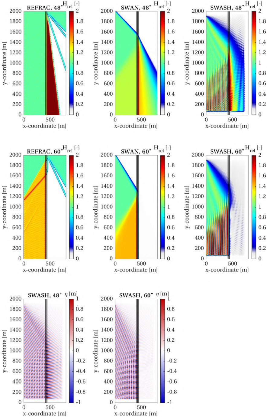
Figure 4.5: First two rows: Relative wave heights  $H_{rel}$  [-] of REFRACT, SWAN and SWASH for waves travelling from shallower towards deeper water, with  $\theta = 48^\circ$  and  $\theta = 60^\circ$  ( $318^\circ\text{N}$  and  $330^\circ\text{N}$ ). Bottom row: SWASH surface elevation  $\eta$  [m] for both angles of incidence.
