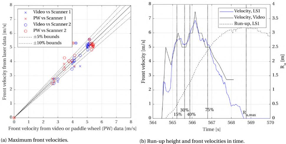
Figure 5.6: Left: Front velocities from laser data compared to video and paddle wheel (PW) data. Right: Run-up and front velocity time signals of one of the laser scanners and front velocity time signal from video analysis for a wave with a filling level of 5 m of test 1. Dotted lines indicate percentages of the maximum run-up level.
