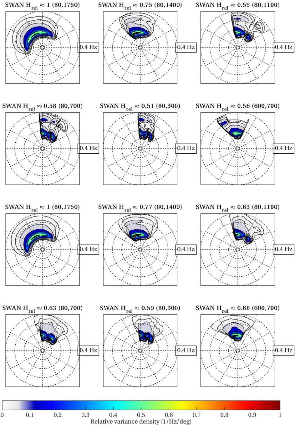
Figure 4.18: 2D SWAN spectra at several locations. First two rows: SWAN with recommended settings, without wind imposed. Bottom two rows: SWAN with recommended settings, with wind. Variance density normalised and colour-scaled with the maximum variance density at the offshore (80,1750) location.
