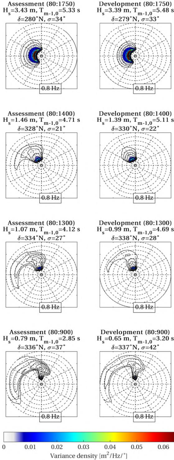
Figure 3.11: 2D spectra for the case with a 1:10 west-east slope, using both the SWAN assessment and development versions.
