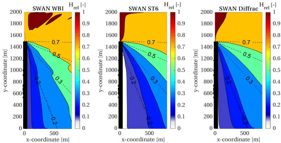
Figure 4.13: Diffraction for semi-infinite breakwater case with irregular, broad-spread waves. SWAN with WBI settings (left), SWAN with ST6 settings (middle) and SWAN with recommended settings, diffraction approximation and 20 m grid cells (right). The black dashed lines indicate the analytical solution of Goda et al. (1978), the thick black line indicates the dike.
