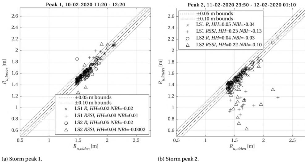
Figure 7.9: Run-up heights above 4.4 m+NAP for both storm peaks for both laser scanners (LS1 and LS2), based on distance  $R$  and laser reflectance  $RSSI$ , compared with run-up heights from video recordings. Left: storm peak 1. Right: storm peak 2. The legend provides the HH and NBI values.
