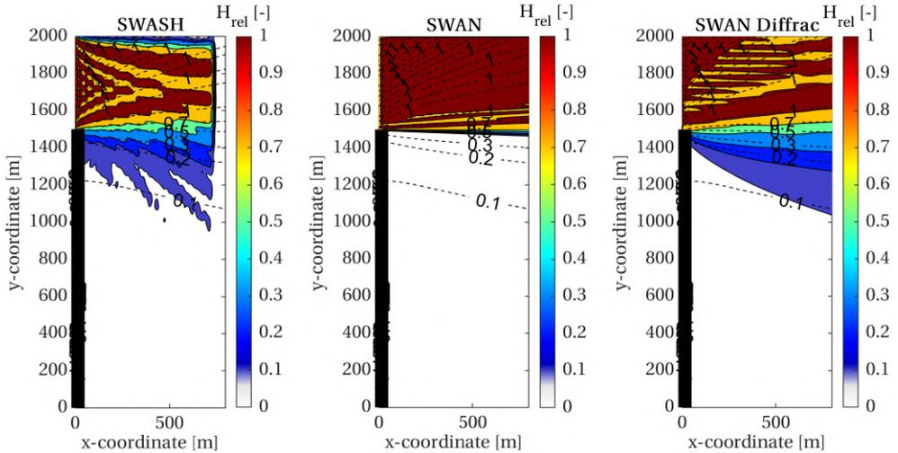
Figure 4.7: Diffraction for semi-infinite breakwater case with regular waves coming from 270°N. SWASH (left), SWAN (middle) and SWAN with diffraction approximation enabled (right), compared to analytical solution of Penney et al. (1952); Sommerfeld (1896) (black dashed lines). The thick black line indicates the dike.
