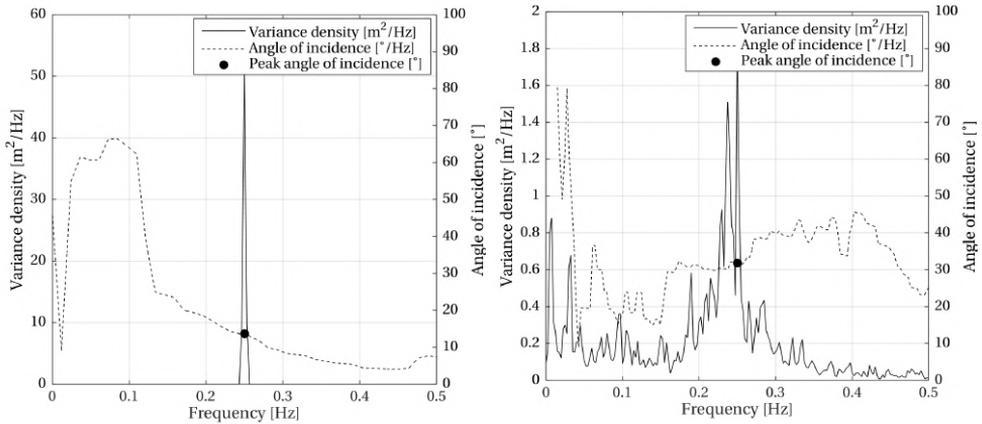
(a) Variance density and angle of incidence spectra, monochromatic waves. (b) Variance density and angle of incidence spectra, irregular, short-crested waves.
