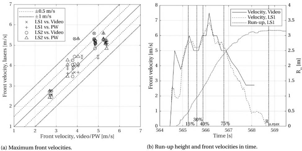
Figure 6.7: Left: Front velocities determined from laser scanner data versus paddle wheel (PW) and video data. Velocities based on front travelling from one paddle wheel to the next. Right: Run-up (dash-dot) and front velocity (dashed) time signals of laser scanner 1 and front velocity time signal (solid line) from video analysis for a single wave. The dotted vertical lines indicate percentages of the maximum run-up level.
