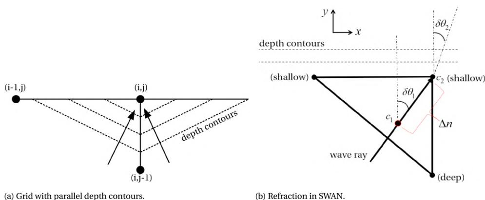
Figure B.1: Left: Geographic grid with parallel depth contours, after [Booij \(1998\)](#). Right: SWAN refraction situation sketch. Definitions of variables given in the main text. Figure after [Zijlema \(2020\)](#).
