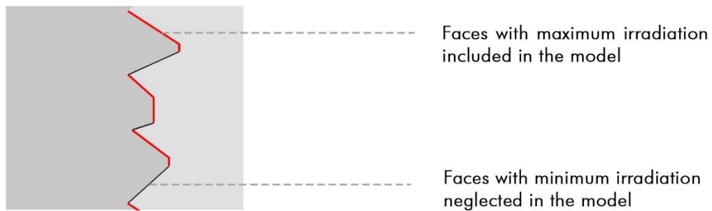
Figure 91 Faces of the facade panels included and excluded in the evaluation model are highlighted
