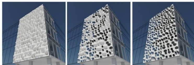
Figure 27 Perspective and elevation of the panels by elimination of low irradiation zones from the panel
