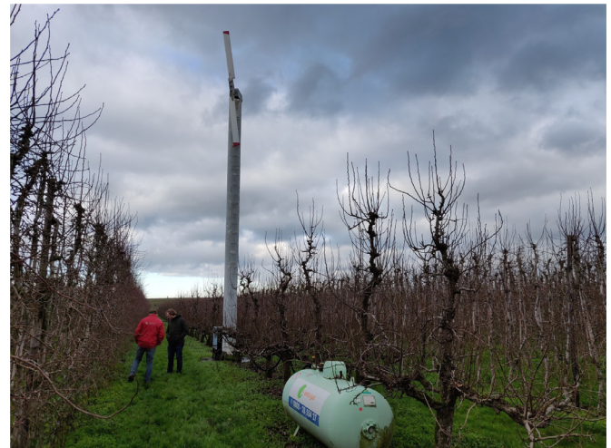
Fig. 2. The wind machine in the pear orchard, with the engine mounted at the bottom of the tower. In the back, the dike is visible.
