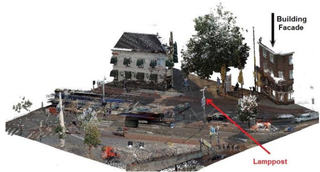
Figure 5. MLS point cloud of an urban scene enriched with RGB (source: Cyclomedia, the Netherlands)
