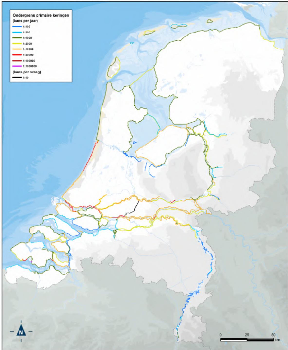
Figure 2.2: Overview of the minimum safety standards in the Netherlands (Slootjes and Van der Most, 2016a)
