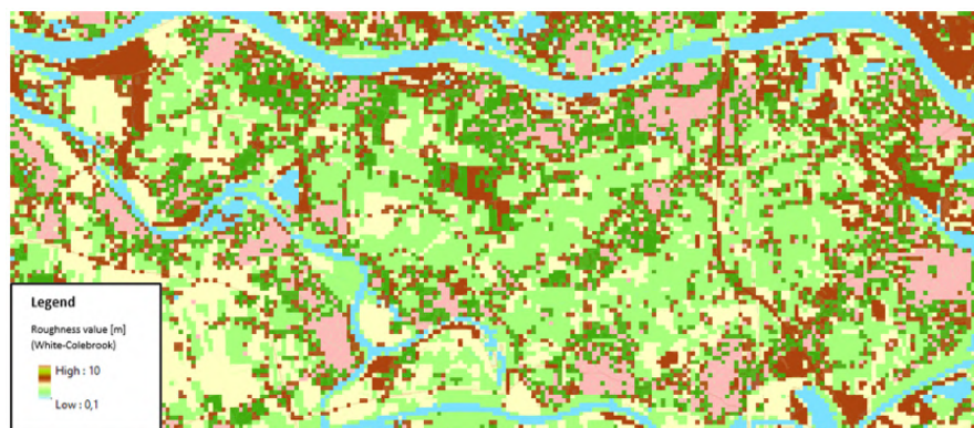
Figure 4.7: Overview of the White-Colebrook roughness values for the 100m resolution model (aggregated from the 25m resolution model)
