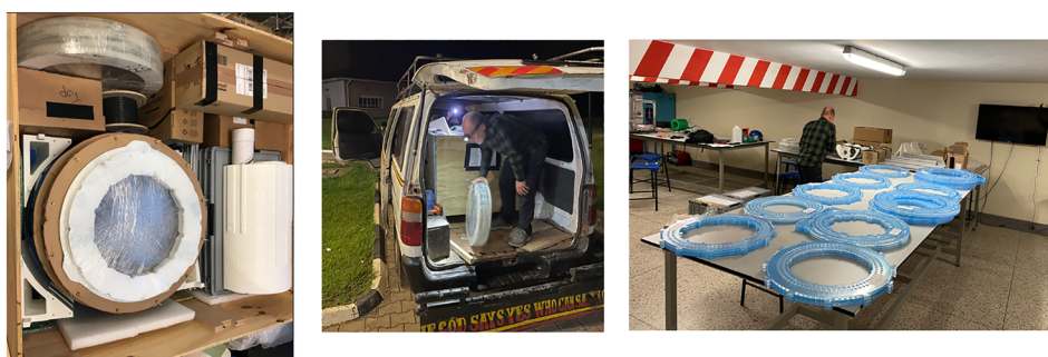
FIGURE 2 Left, Crate containing all components including assembly tools, overall size 1.2 \text{ m} \times 1.0 \text{ m} \times 0.8 \text{ m} and weight 325 kg. Center, Final delivery after two weeks en route, via taxi from the closest airport 5 h away. Right, Illustration of individual plastic rings for the magnet.
