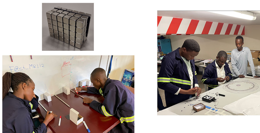
FIGURE 3 Individual steps in preparing the magnet components. Cubic magnets (upper left) are coloured to indicate north/south poles (lower left), and magnets are inserted manually into the holes in each ring (right).
