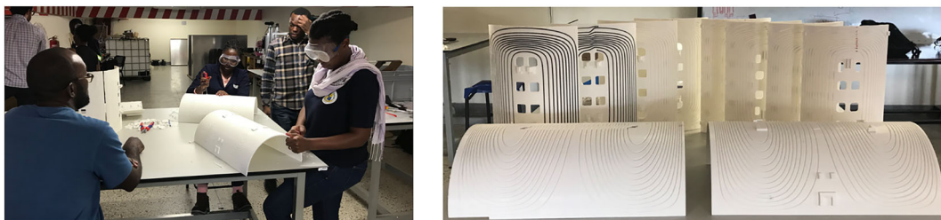
FIGURE 6 Stages involved in gradient coil assembly from 3D printed formers. Left, Residual plastic from the 3D printing is removed to clear the grooves. Insulated wire is placed into the grooves and superglued into place after each turn. Right, Photograph showing one completed section: four sections are used for the two outer gradient sets, and two sections for the inner set.
