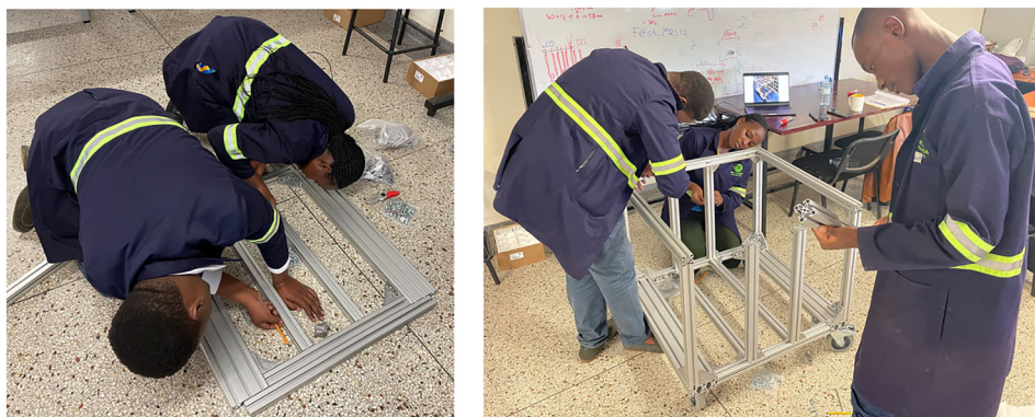
FIGURE 8 Construction of the portable trolley used for the system. Components consist of aluminum subunits screwed together.
