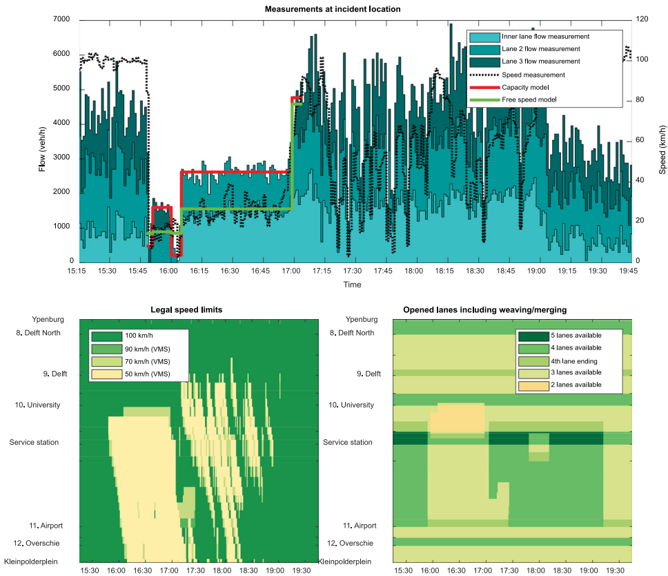
Figure 10. A13 flow at crash location and applied traffic control.
