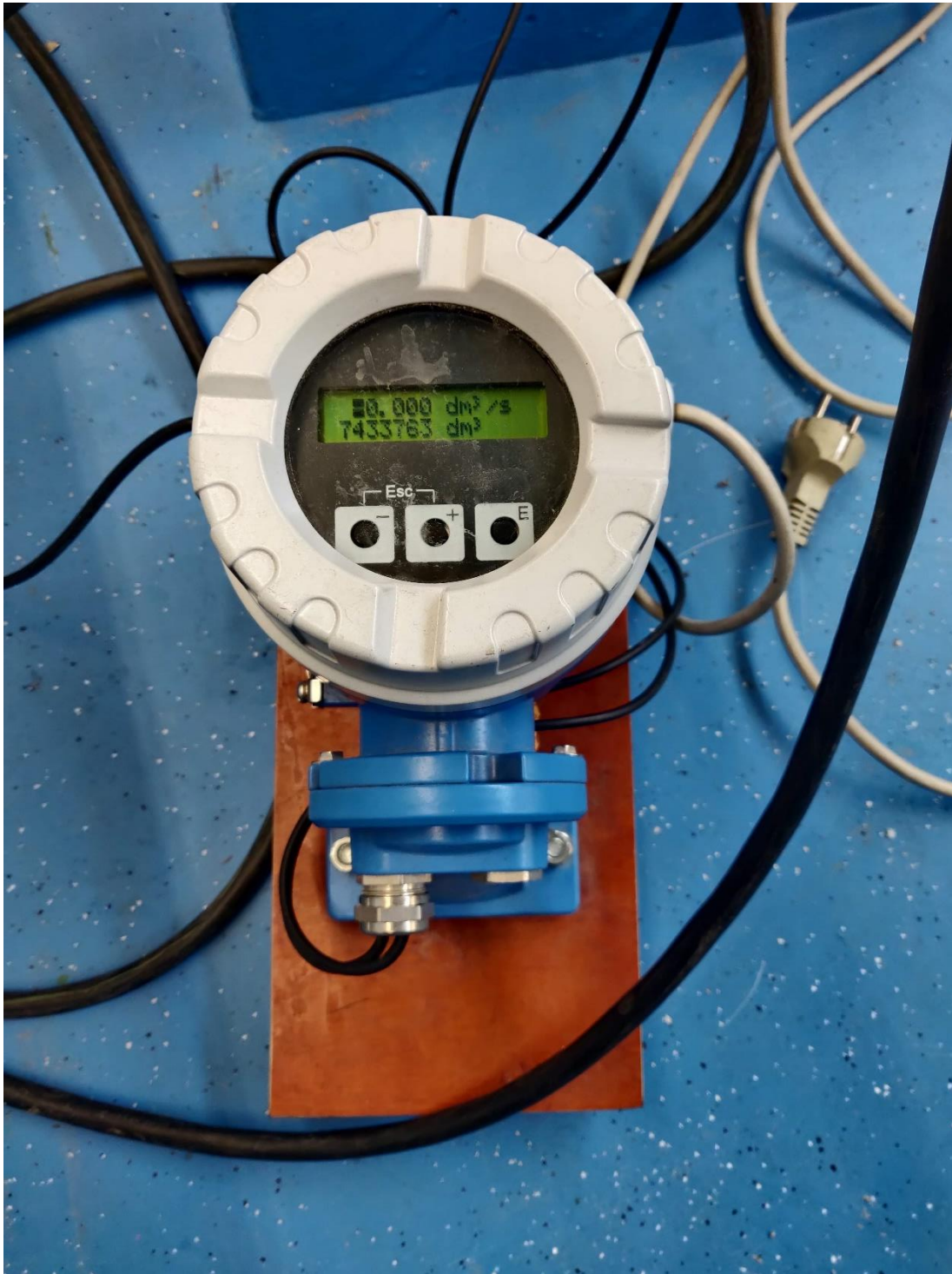
Figure 14 The flowmeter. It is connected to both the pipe and the computer. Discharge data was collected by reading it directly off the flowmeter.
