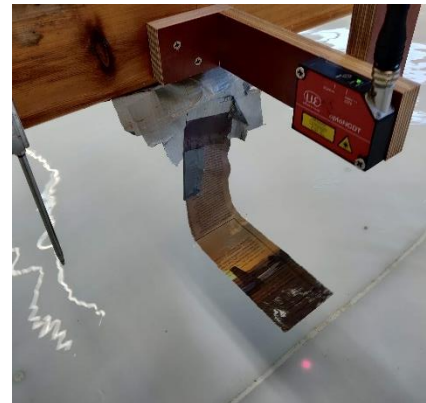
Figure 8 The setup for the laser. It only works if the paper reflects the laser, in other words when the water level is high enough.
