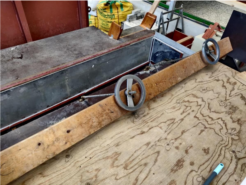
Figure 16 Gate to set the downstream water level.
