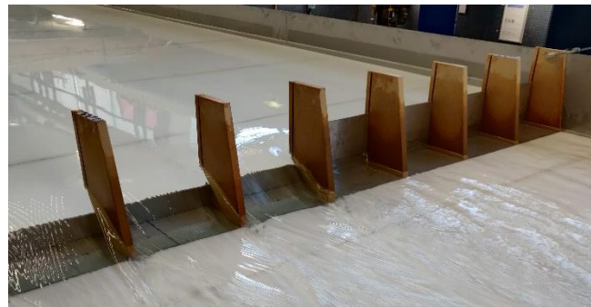
Figure 7 The experimental setup with buttresses and panels. The model consists of 12 gates. Each gate can be configured individually.
