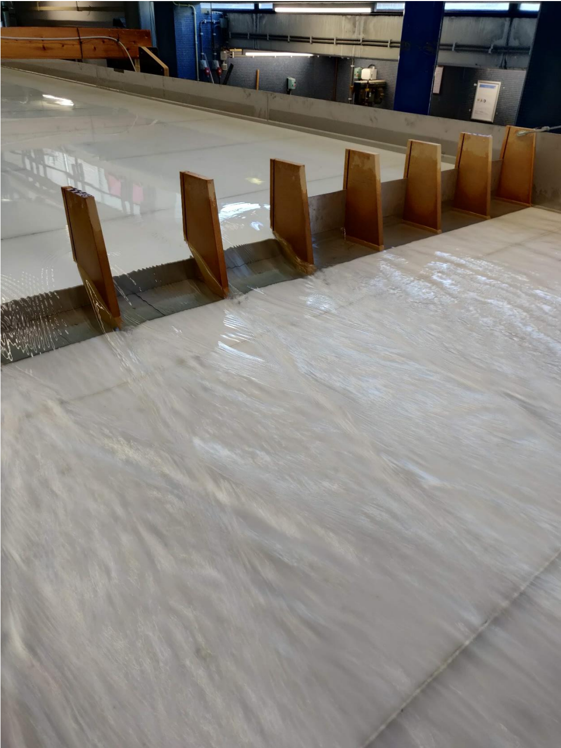
Figure 17 The buttresses and the gates with a super critical flow.
