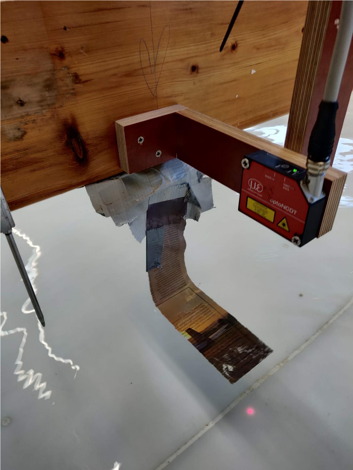
Figure 18 Setup to measure the water levels. It consists of a laser that is reflected by a piece of paper floating on the water.
