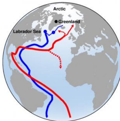
Figure 1.1 Schematization of the Atlantic Meridional Overturning Circulation (AMOC). In the upper layers, relatively warm waters flow northwards (red). In deeper layers, cold waters return southwards (blue). Deep convection zones are highlighted with the blue dots (Irminger Sea and Labrador Sea). From: The National Oceanography Centre (2018).
