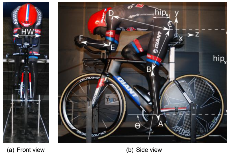
Figure 6.1: Cyclist model and bike with characteristic dimensions. Duplicated from (Terra et al., 2016a).
