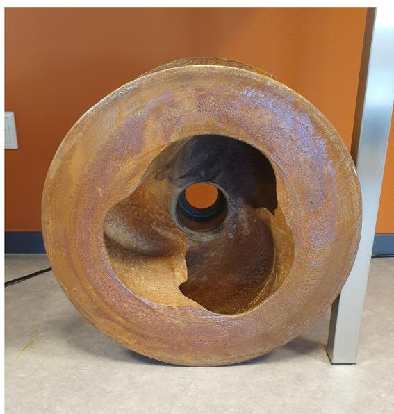
**Figure 1.1:** Example of a severely eroded impeller
