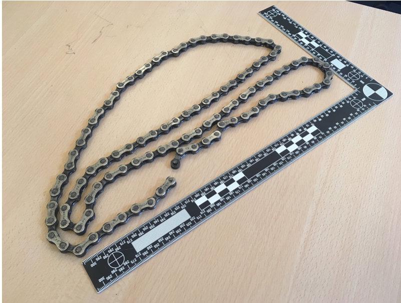
Fig. 4 Example failed bicycle chain.
