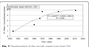
Fig. 2 Development of the aircraft speed over time [35]
