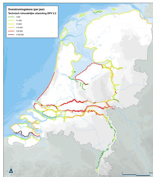
Figure 1. Proposed new flood protection standards in terms of maximum acceptable failure probability of embankment stretch [17, 22]
