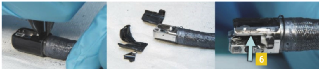
c. trimming the tip cover
