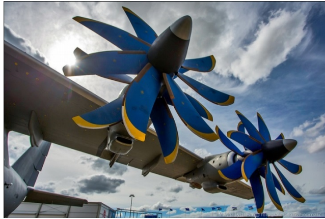
Figure 1.2 An example of contra-rotating propellers implemented on the Antonov An-70 aircraft. ([30])
