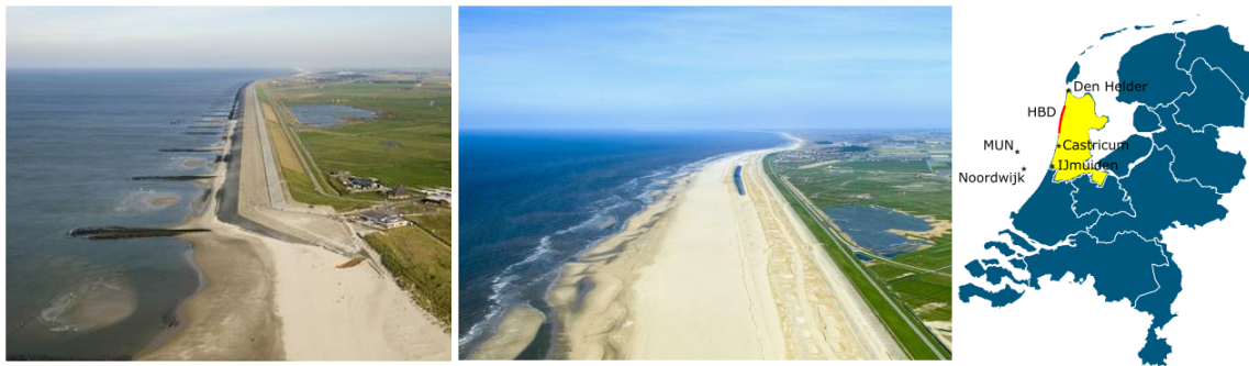
Figure 2: Hondsbossche and Pettemer Zeewering, a sandy coastal flood protection near Petten, the Netherlands. The original, hard protection in 2005 (left) and the new sandy coastal protection in 2015 (right).
