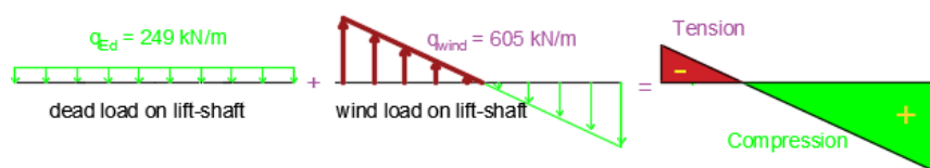
Figure 53: tension in the foundation due to wind
