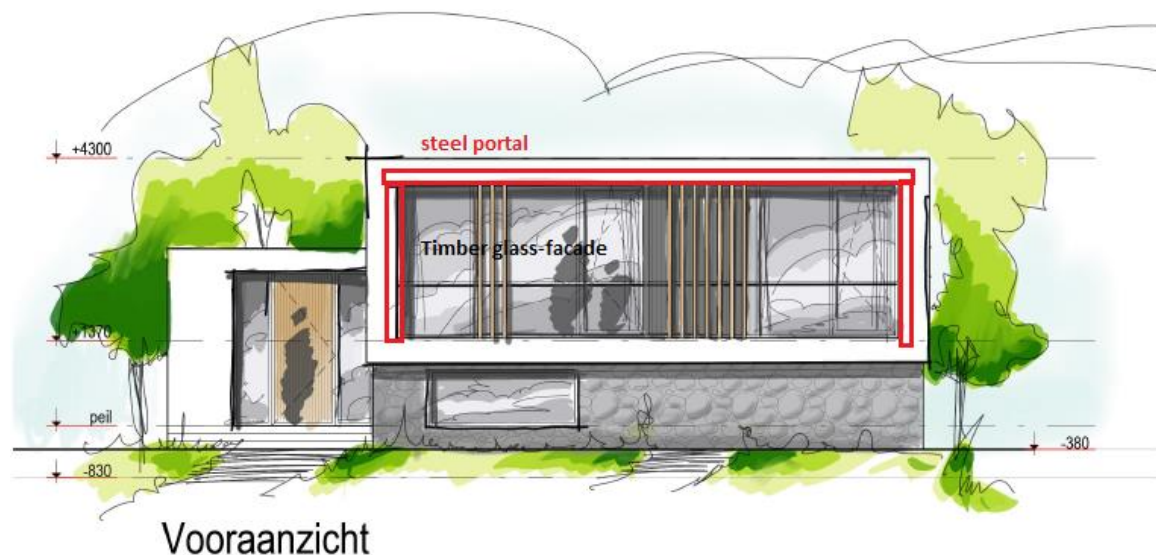
Figure 25: expansion building with steel portal and glass façade
