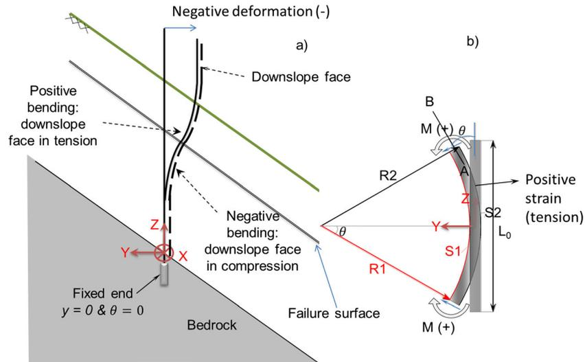
**Fig. 11** Slope deformation sensors. **a** Coordinate system and sign convention. **b** Initial condition and deformed shape
