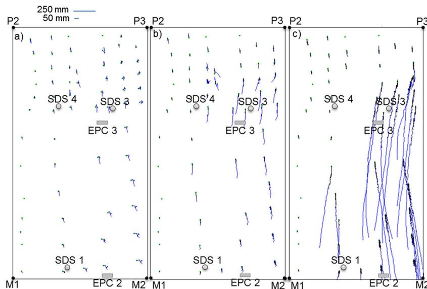
**Fig. 10** Displacement of the target points on the slope surface. a Between the start of sprinkling and 23 min before failure. b During the last 22 min before failure. c During failure. (Locations of M1, M2, P2 and P3 are shown in Figs. 1, 2 and 3)
