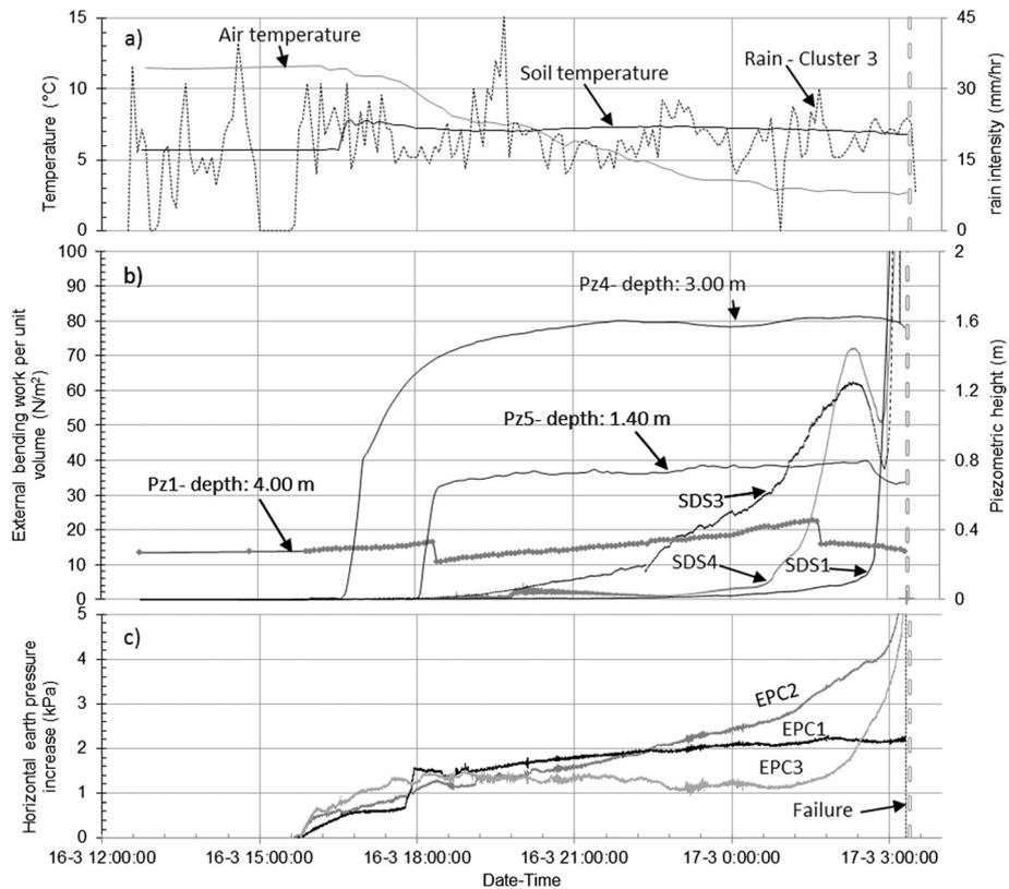
**Fig. 14** a Rainfall measured at cluster 3, soil temperature at 60 cm depth at cluster 2 and air temperature measured at the upper part of the slope. b External bending work per unit volume of slope deformation sensors and Piezometer measurements. c Changes in horizontal earth pressure
