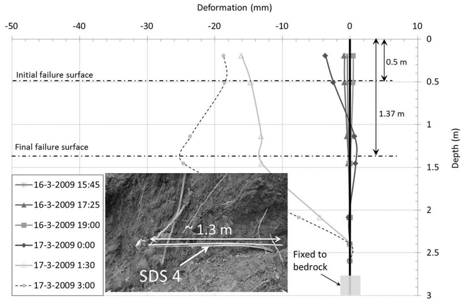
**Fig. 13** Deformation profile of SDS4 during the landslide triggering experiment. The small photo on the lower part of the graph shows the deformed SDS after failure
