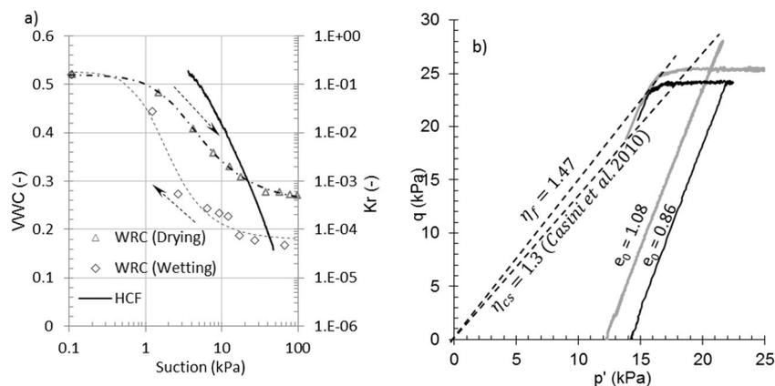
**Fig. 4** a Water retention curve (WRC) of natural undisturbed samples from the test site determined using the axis translation technique and hydraulic conductivity function (HCF) for reconstituted Ruedlingen soil, derived with the instantaneous profile method (VWC volumetric water content). b Stress paths during consolidation and shearing of specimens in unsaturated constant shear triaxial tests
