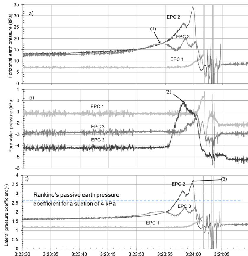
**Fig. 15** Data measured at a depth of 0.6 m in all three clusters during the last 40 s of experiment before landslide. **a** Horizontal soil pressure. **b** Pore water pressure. **c** Horizontal earth pressure coefficient
