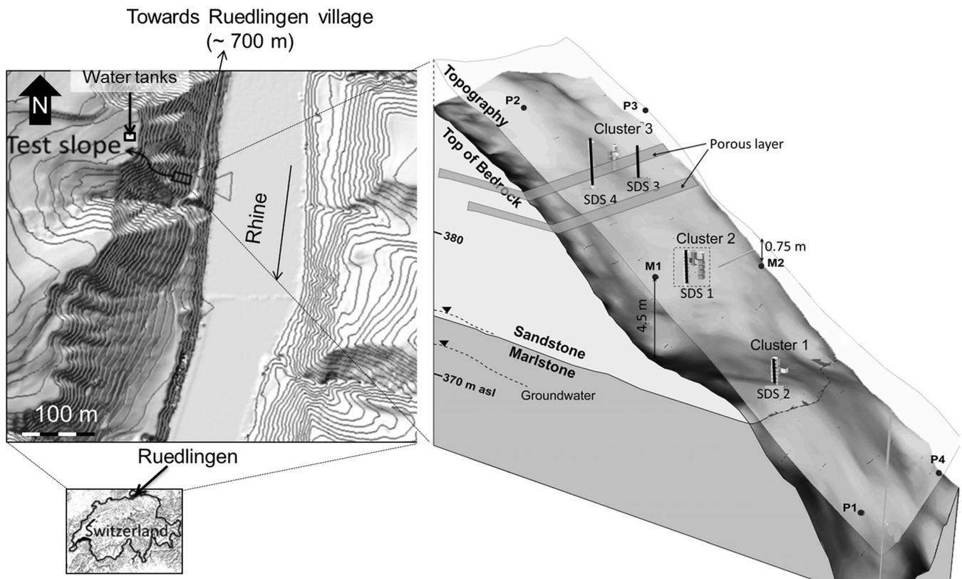
**Fig. 1** Left: The location of the test slope and topography of the region (The interval between elevation contours is 5 m. The relief and topography map is taken from <http://www.sh.ch/>). Right: Shape of the bedrock, positions of the sensor cluster and the slope deformation sensors (after Brönnimann 2011)
