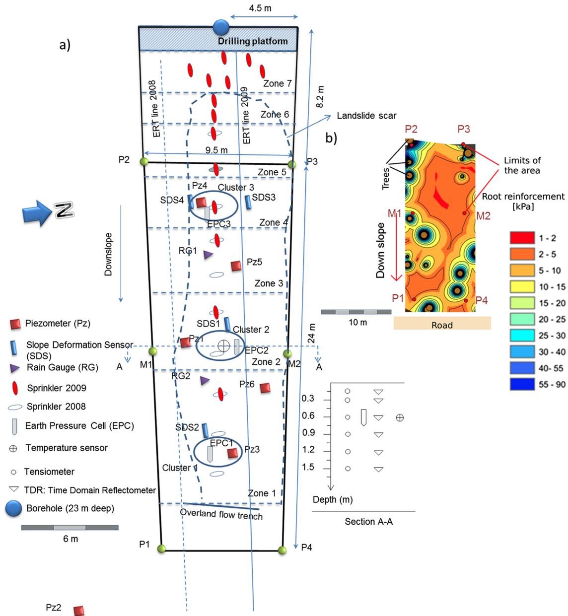
**Fig. 3** a Instrumentation and different raining zones in the Ruedlingen test site; ERT electrical resistivity tomography (after Askarinejad 2013). b Spatial distribution of maximal root reinforcement in the study area (after Schwarz 2011). The instrumentation arrangement as shown in cross section A-A is also applied to other instrumentation clusters
