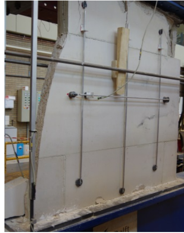
(c) CS element masonry failure mode
